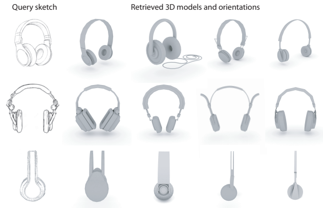
Figure 10: Results from our 3D shape search engine. Even though the searched models had no ground truth correspondence on the model database, our algorithm returned plausible shapes. Our features additionally provide information about the sketch view, allowing to automatically orient models to the query sketch.
