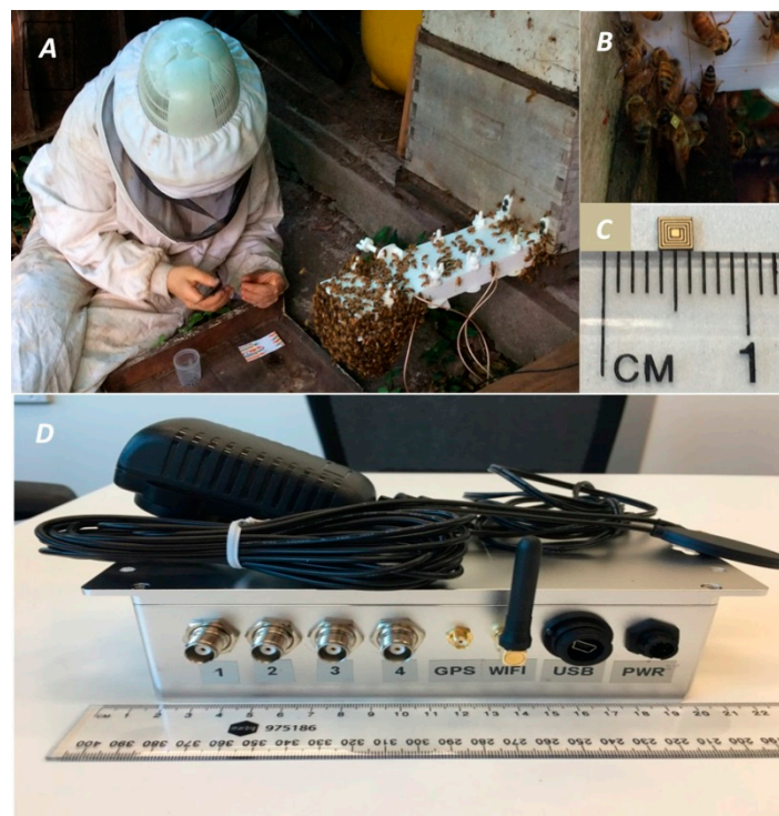
Figure 2. (A) Drones being tagged beside the hive. The white box at the entry is where the two pairs of patch-type RFID antennas are located. (B) Drone fitted with RFID microchip. (C) RFID microchip (Tag). (D) Reader unit with four connectors visible (one for each RFID antennas, Wi-Fi antenna, GPS connector and data and power connectors). A full description of this system is provided at [25].
