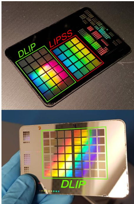
Fig. 5 Photographs of LIPSS and DLIP treated samples (as labeled in the figure) showing the structural coloration.
