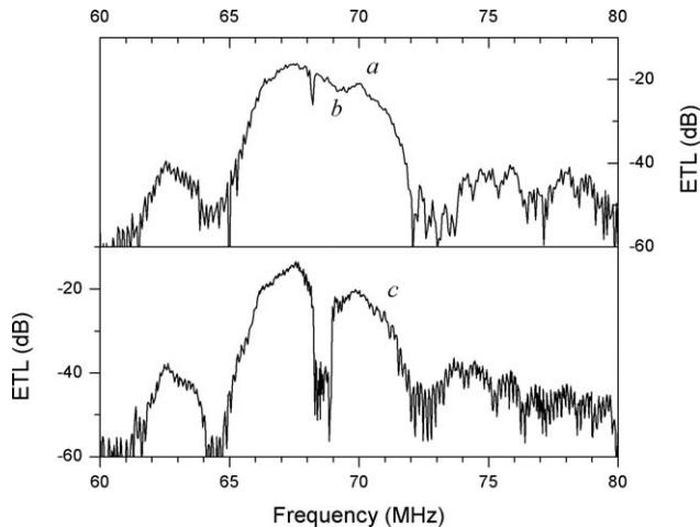
**Figure 2** Effective transmission loss of laser fabricated two-port SAW device with free surface (a), 1D (b), and 2D (c) PC structures
