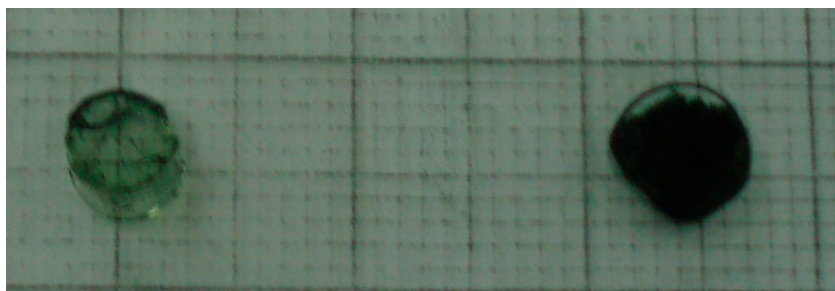
Figure 1. Photographs of poly( N -isopropylacrylamide) (PNIPAM) (with 2% 2-acrylamido-2-methyl-1-propanesulfonic acid (AMPS)) hydrogels after immersion in a dispersion of polyaniline (PANI) nanofibers. The nanoporous hydrogel ( left ) was made by polymerization at ambient temperature, where the macroporous hydrogel ( right ) was made by polymerization using cryogelation ( -20\text{ }^{\circ}\text{C} ). Then, both were exposed to a dispersion (1% p/v) of PANI nanofibers in water. Both gels were exposed to 700 W of microwave radiation by 30 s.
