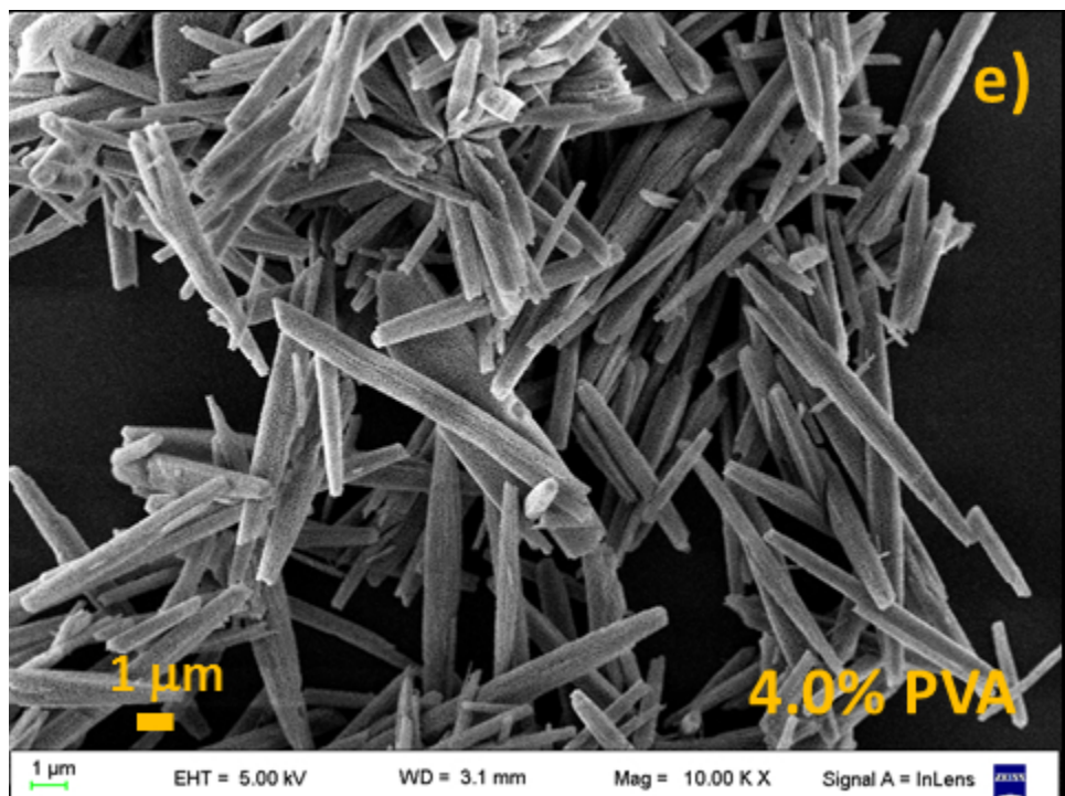
FIG. 2 CoFe 2 O 4 particles synthesized with different amounts of PVA after calcination. (a) 0.0 %, (b) 1.0 %, (c) 2.0 %, (d) 3.0 %, (e) 4.0 % and (f) 5.0 % w/w.
