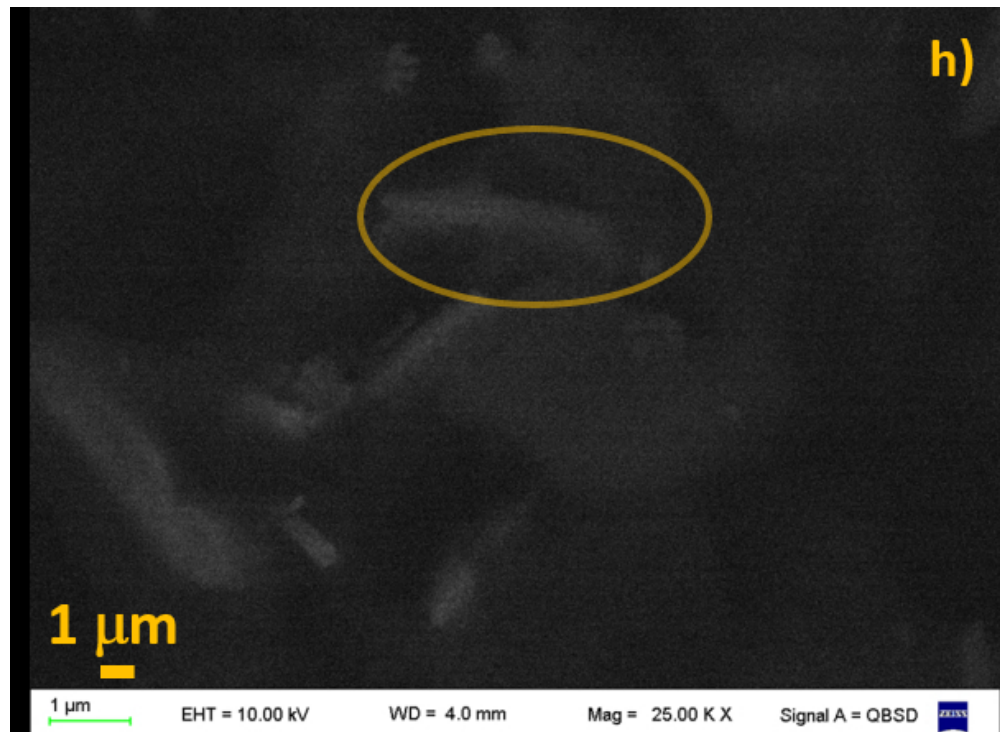
FIG. 8. Typical SEM images of CoFe 2 O 4 nanorods-PANI of different feed compositions: (a) and (b), rS = 6; (c) and (d), rS = 12; (e) rS = 20; (f), (g) and (h), rS = 16. In image pairs (a) - (b), (c) - d), and (g) - (h) the same region of the sample was imaged with two different detectors: InLens in and QBSD, respectively. The same particle is encircled in each case for better comparison.
