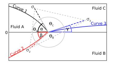
FIG. 2. Contact angle definitions for a liquid lens (fluid A) over a deep liquid substrate (fluid B), surrounded by air (fluid C).
