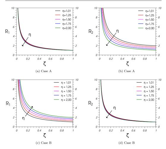
FIG. 6. Solution without gravity: Radius of curvature of each surface of the lens as a function of  $\zeta$  for  $\eta = 1.01, 1.25, 1.50, 1.75$ , and 2.00. (a) For curve 1 and (b) curve 2 in case A ( $\sigma_1 < \sigma_2$ ), and (c) for curve 1 and (d) curve 2 in case B ( $\sigma_2 < \sigma_1$ ). The arrows indicate the direction of increasing  $\eta$ .
