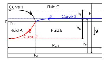
FIG. 1. Dimensionless scheme of a liquid lens (fluid A) over a deep external liquid (fluid B), surrounded by air (fluid C). The triple contact line is at  $r = R_d$  and z = 0 ( $R_d \ll R_{wall}$ ). The arrows over each curve indicate the increasing direction of the arclength, s. The length scale is  $\mathcal{R}_0$  [Eq. (1)].
