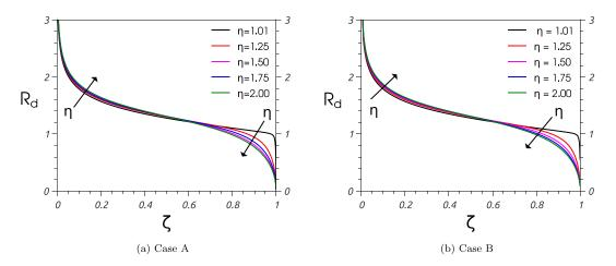
FIG. 5. Solution without gravity:  $R_d$  as function of  $\zeta$  for  $\eta = 1.01$ , 1.25, 1.50, 1.75, and 2.00 for cases A ( $\sigma_1 < \sigma_2$ ) and B ( $\sigma_2 < \sigma_1$ ). The arrows indicate the direction of increasing  $\eta$ .
