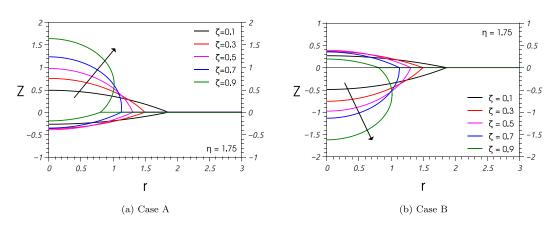
FIG. 4. Solution without gravity: Drop profiles for  $\eta = 1.75$  and  $\zeta = 0.1, 0.3, 0.5, 0.9$  for cases A ( $\sigma_1 < \sigma_2$ ) and B ( $\sigma_1 > \sigma_2$ ). Note that the free surface of the liquid substrate (curve 3) is flat for all  $\zeta$ .
