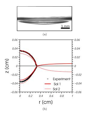
FIG. 14. (a) Experiment: Silicon oil (PDMS) drop on water (case A with  $\eta = 1.79$  and  $\zeta = 0.04$ ). (b) Comparison of drop shape with solutions Sol 1 and Sol 2.
