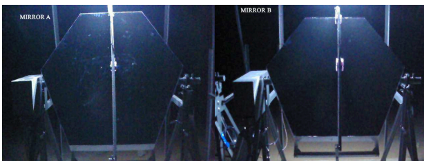
Figure 5: Mirrors surface captured by the IP Camera during the night of May 12th, 2013. No features due to icing or condensation are seen in the images. Left: Mirror SACK010-0213 (A). Right: Mirror SACPNG01-0213 (B).
