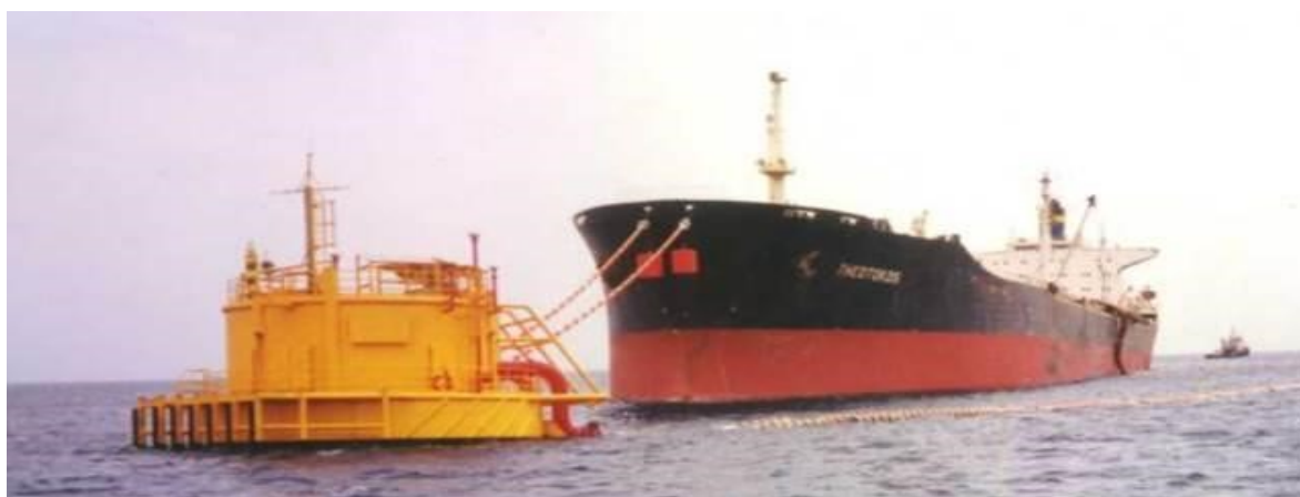
Figure 2. CALM Buoy with an FSO offloading tanker off the shore of Sudan (Courtesy of Bluewater).
