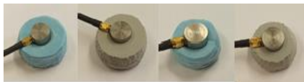
Figure 2. Foam holders left to right: low density / 5.5cm \varnothing , high density / 5.5cm \varnothing , low density / 4.5cm \varnothing , high density / 4.5cm \varnothing .
