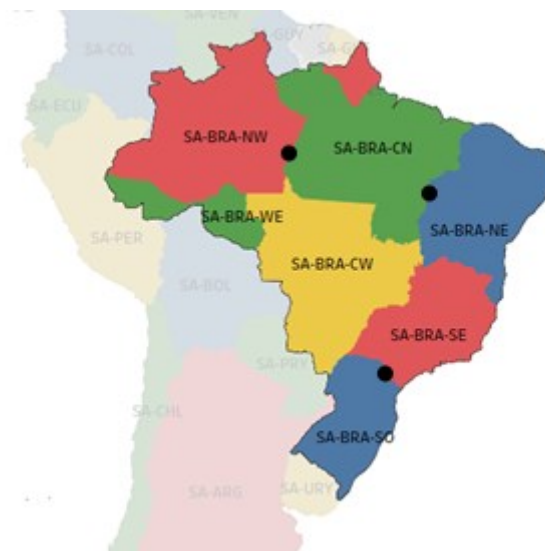
Figure C-2 Nodal representation of Brazil in PLEXOS-World. Every copperplated area of an individual colour represents a node with a total of 10 independent nodes, consisting of 7 nodes with demand and generation portfolios and 3 transmission junction nodes that represent transmission interconnections connecting large hydro facilities with demand centres (indicated with asterisks on the map).
