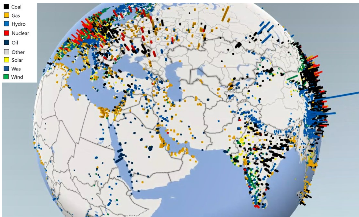
Figure 4-3 Visualization of the power plant data of the WRI database. Relative height of the bar is an indicator for the capacity of the specific power plant.
