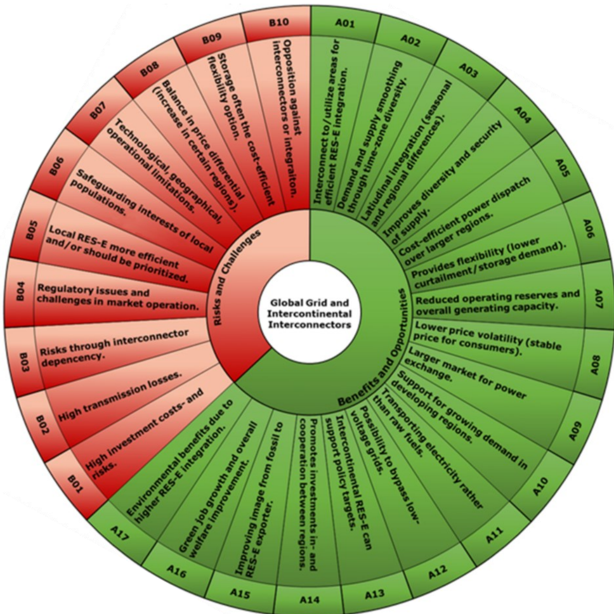
Figure 2-2 Overview of mentioned benefits, opportunities, risks and challenges for the global grid concept within the literature. The outer ring corresponds to further description of the benefits and opportunities (A) and risks and challenges (B) within this section.
