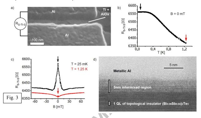
Superconductor (S-TI-S) junctions were consisted of Al evaporated via shadow mask on top of an Al-
