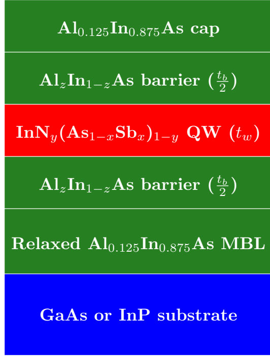
FIGURE 4.2: Schematic illustration of the structures considered to design strain-balanced \text{InN}_y(\text{As}_{1-x}\text{Sb}_x)_{1-y}/\text{Al}_z\text{In}_{1-z}\text{As} QW LED devices.
