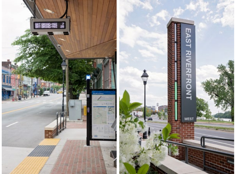
Figure 26: Digital message boards and a light totem indicate when the next bus will arrive.
