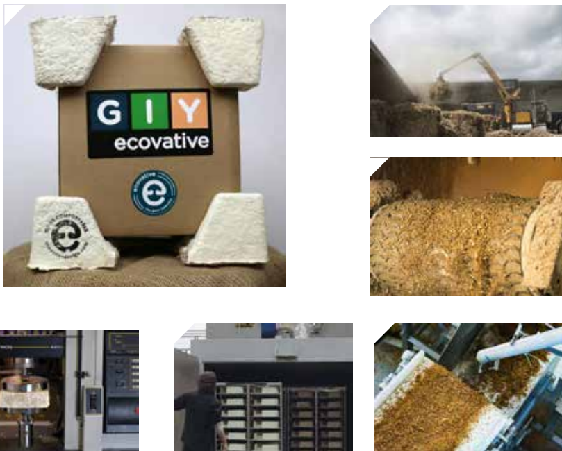
Figure 4.5 Production of Mycofoam™ from agricultural waste, showing the raw material, inoculation by a fungal strain, incubation and pressing. The example shows protective corner mounts, replacing the use of EPS; images courtesy of Ecovative.
