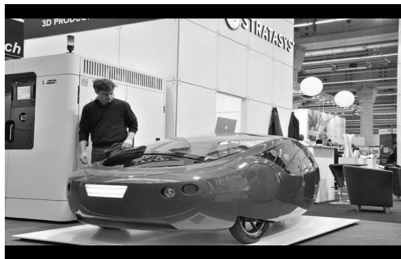
Fig. 5. The first car, manufactured by means of the 3D-printer
