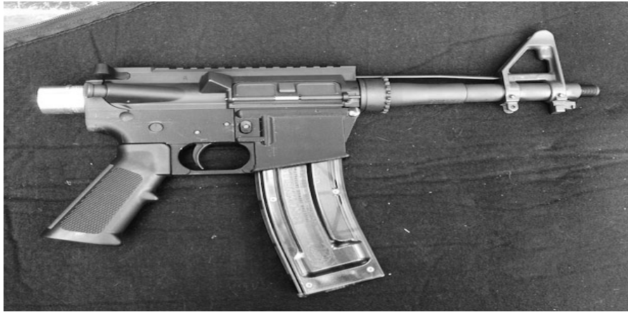
Fig. 6. Gun, manufactured by 3D-printer
