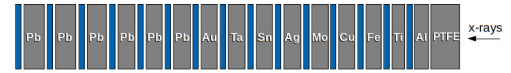
FIG. 1: Schematic disposition of the filters (in grey) and imaging plates (in blue). X-rays are penetrating the stack from the right.
