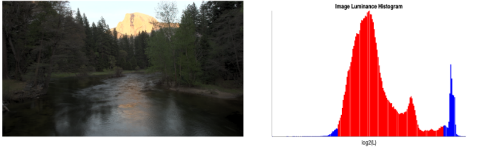
Figure 2.11: Example image tone-mapped using Optimal Exposure [Debattista et al. , 2015]. Left. HDR Tone-mapped image, bit-depth: 8 bits. Right. Histogram of the log-luminance values, red indicates the range selected by the algorithm, blue indicates the information discarded due to the specified bit depth. Image courtesy of Fairchild [2007b].
