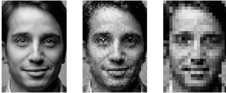
Figure 3.1: Examples of facial images with different quantisation. From left to right: full resolution (over 500 pixels/face), 26 pixels/face, 18 pixels/face.
