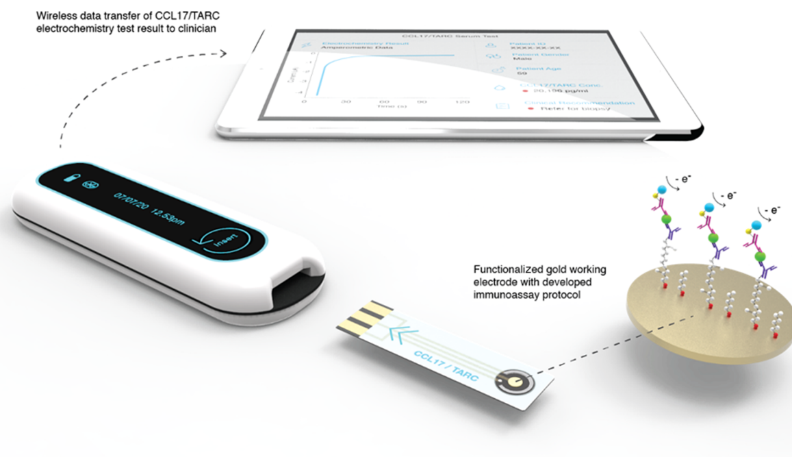
Figure 1. Product concept for the proposed electrochemical sensor and overview of the developed sandwich immunoassay.
