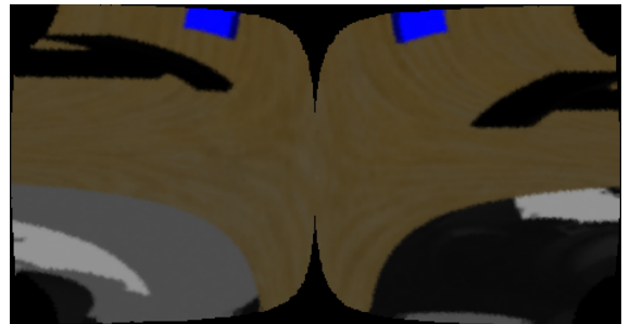
Fig. 6. Cortical image generated by software retina using image from the in-wrist camera.
