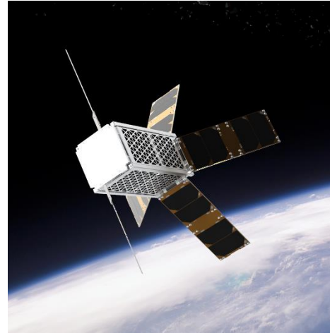
Fig 3. Render of STRATHcube in the 'Shuttlecock' Configuration for Atmospheric Re-entry
