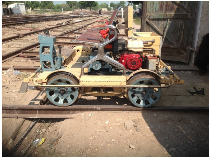
Figure 4. Mechanical railway cart used for data collection. The cart is driven by the engine that is manually controlled.
