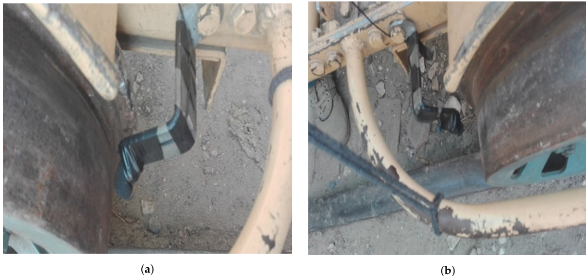
Figure 5. Pictures of wheels in contact with the track. (a) Assembly of microphone on left side of the mechanical cart; (b) Assembly of microphone on right side of the mechanical cart.
