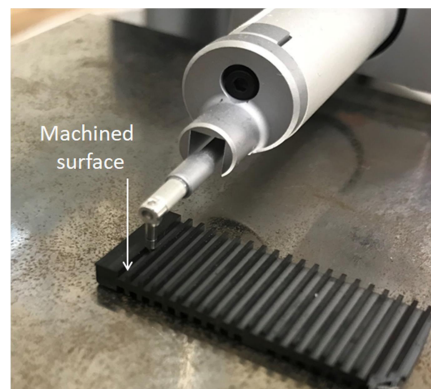
Figure 3.21: Surface roughness Ra measurement using Mitutoyo SJ-410 contact style profilometer
