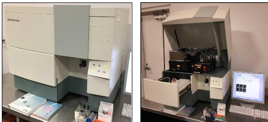
Figure 1-2 Image of a BD FACSCalibur Calibur Flow Cytometer 4 Color [from https://images.app.goo.gl/x1LYbPvzsEEgJGEB7 ]. The flow cytometer is costly, bulky, requires electricity and refrigerated reagents and a skilled operator for its operation and maintenance.
