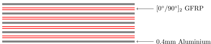
Figure 5.1: Specimen 7, GLARE, cross section.
