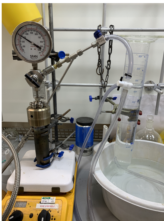
Figure 4.16: Experimental set-up used to carry out high pressure CO 2 measurements. Consists of a 75 mL Parr vessel with pressure gauge and connected to an inlet for 50 bar CO 2 and an outlet to capture the gas in an inverted measuring cylinder.
