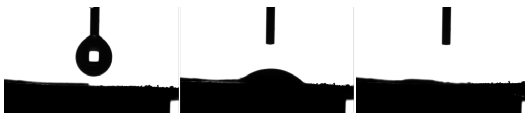
Figure 4.13: Frames from video recording of dropping water onto the 'knitted' benzene HCP, where the water is fully absorbed by the droplet, in the third frame a small amount of swelling of the pellet can be observed.
