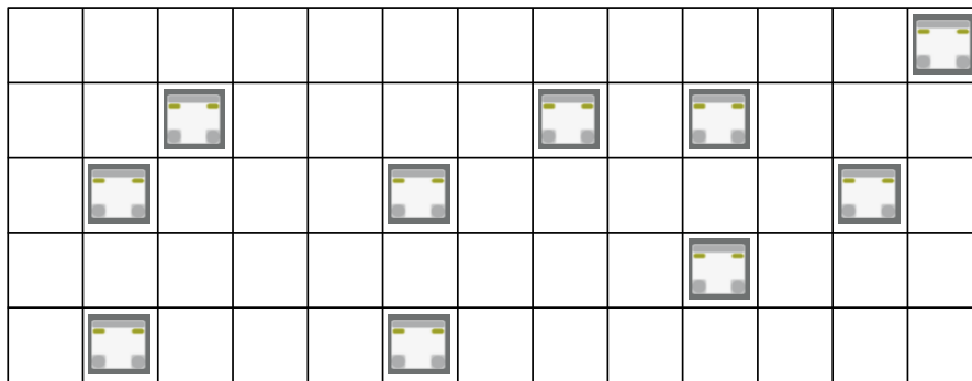
Figure 1.2: A number of robots travel atop a square grid system inside Ocado's warehouses.
