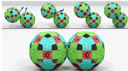
Figure 1.4: Two catoms are shown next to each other at the bottom, while the rotation movement is shown at the top [97].
