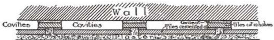
FIG. 52.—Plan of Ventilating (Tile and Plaster) Lining to Interior of Damp Walls.
