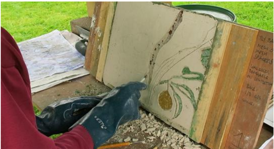
Fig. 25: Test panel 2. Starting to cut using scalpel blade in a handle. Panel moved to upright position. Note plaster residue left on colour layer over tree trunk as main bulk of material removed. It peeled off with little pressure.
