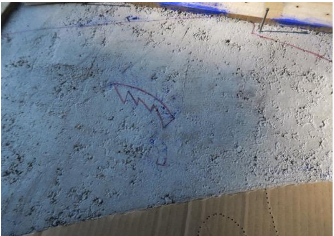
Fig. 34: Test panel 3. Base coat with colour block outlines pounced through with blue colour powder and painted in. Mask for green visible at bottom right.
