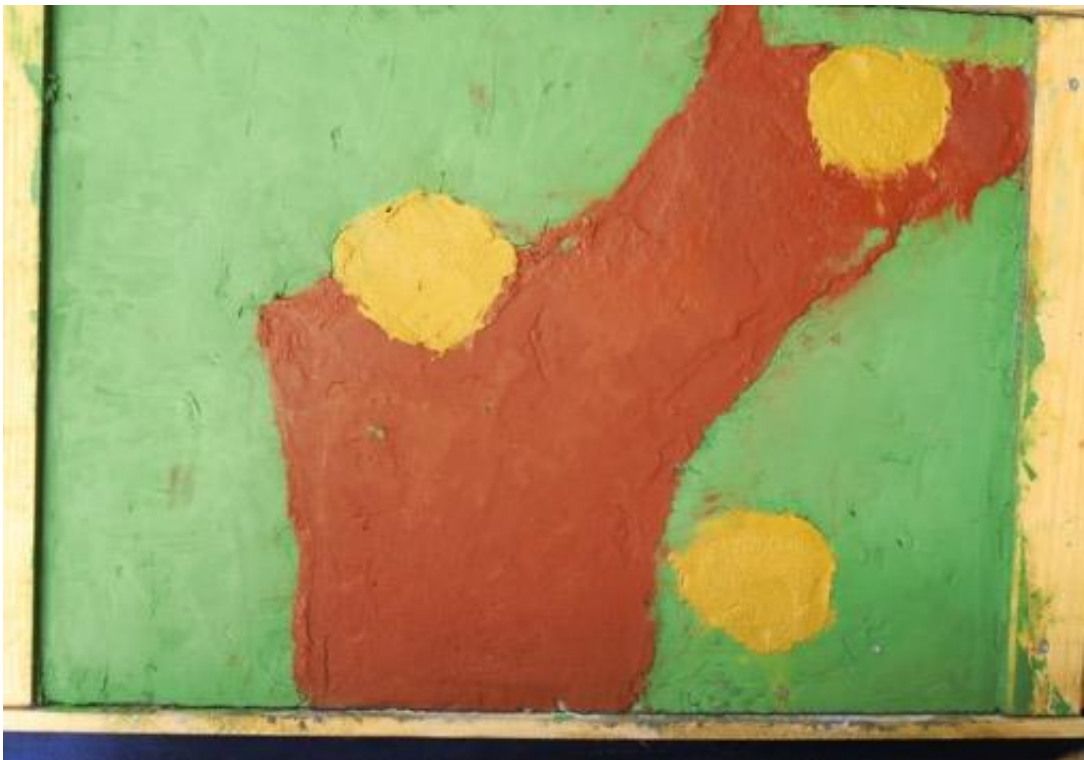
Fig. 22: Test panel 2. Colour blocks in place. Wetting of the base coat did not occur for the application of the green and this began to dry and crack very quickly. Extensive repeated wetting and working over the surface was needed to mitigate this failure in the process.
