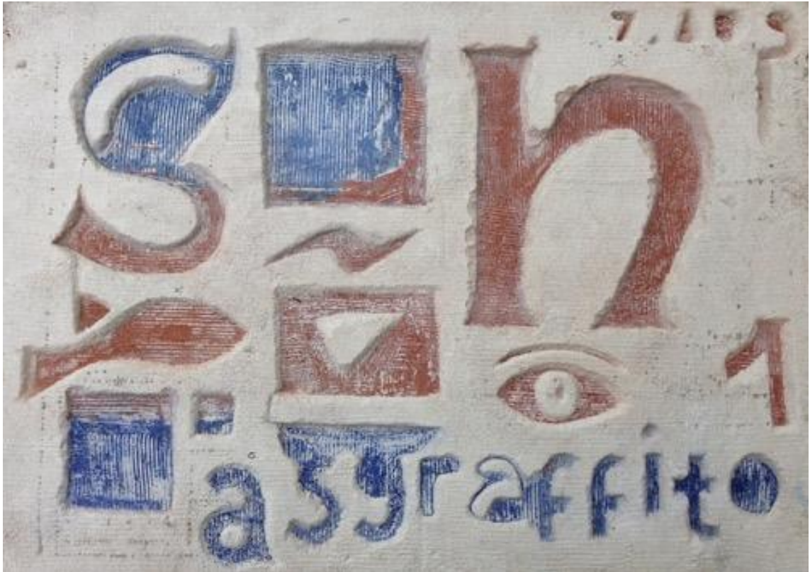
Fig. 18: Test panel 1, completed. The group of shapes across the middle of the panel, from left to right, fish; triangle in square; eye and brow, figure '1' and at top right a notional date, were cut in the 'tough' stage using a combination of scalpel and pointed but round ended metal-working tool.
