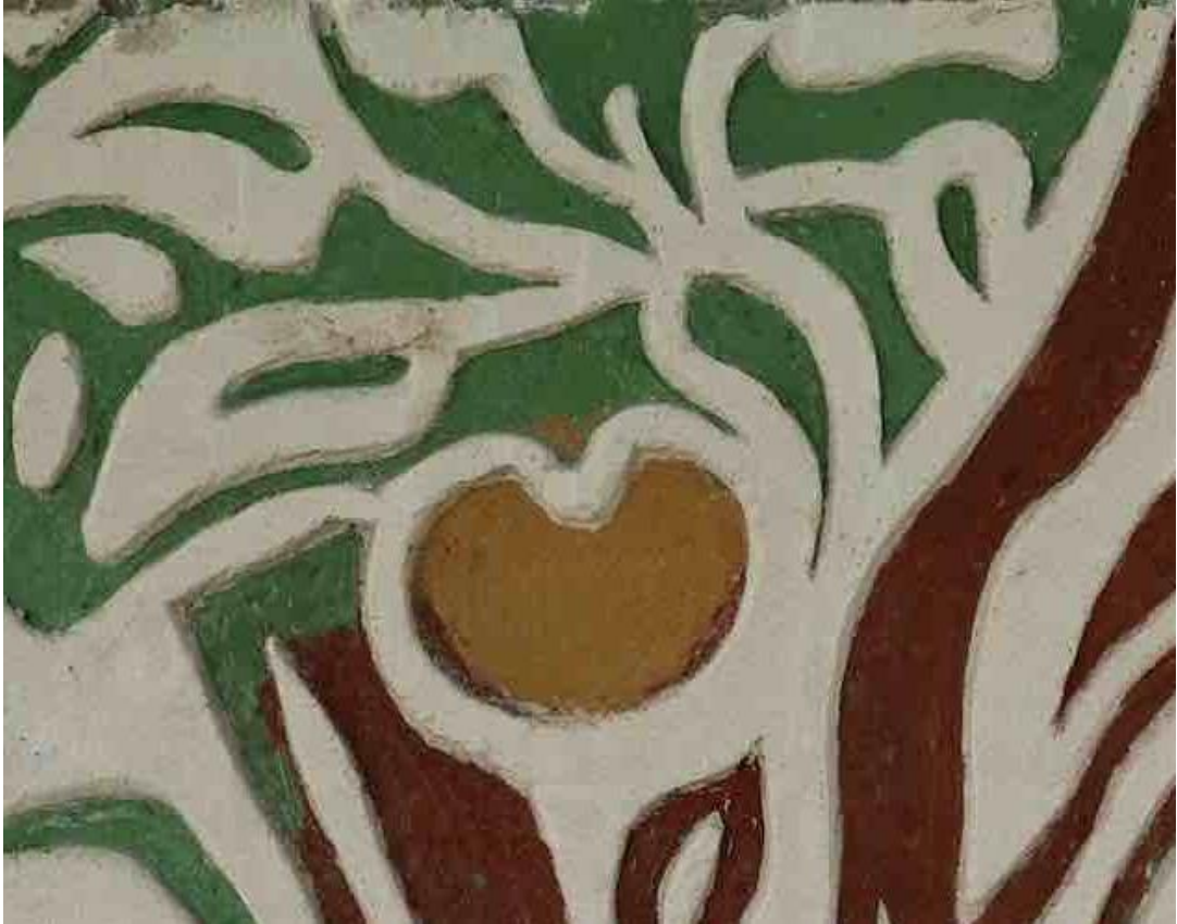
Fig. 30: Test panel 2. Enlarged detail of completed panel. Scraping of colour coat can be seen as can the repair near the centre top. Such working marks are visible in Sumner's sgraffito upon close inspection.
