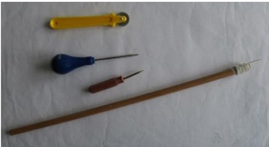
Fig. 7: The various tools tried for pricking through designs. The blue handled bradawl was the author's preferred option.
