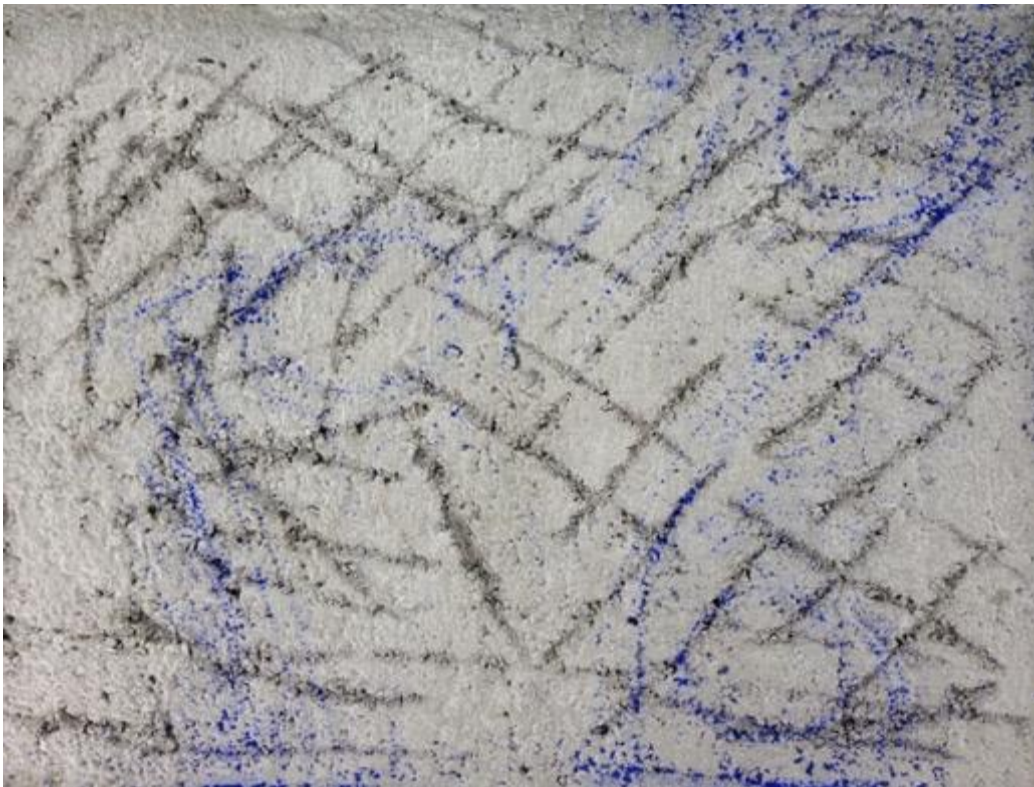
Fig. 20: Test panel 2. Blue powder outline on base coat.
