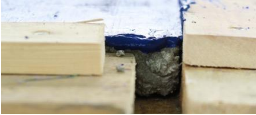
Fig. 11: Test panel 1. Blue colour coat complete. View at gap in frame edges showing thickness and guide battens for depth of later coats.
