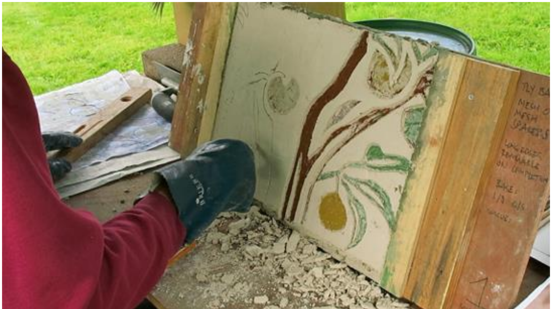
Fig. 27: Test panel 2. Continuing cutting. Note the various stages of cleaning out residue.
