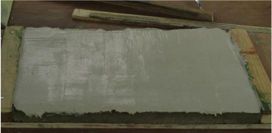
Fig. 23: Test panel 2. Waiting for topcoat to dry sufficiently. Damp sheen is still visible.
