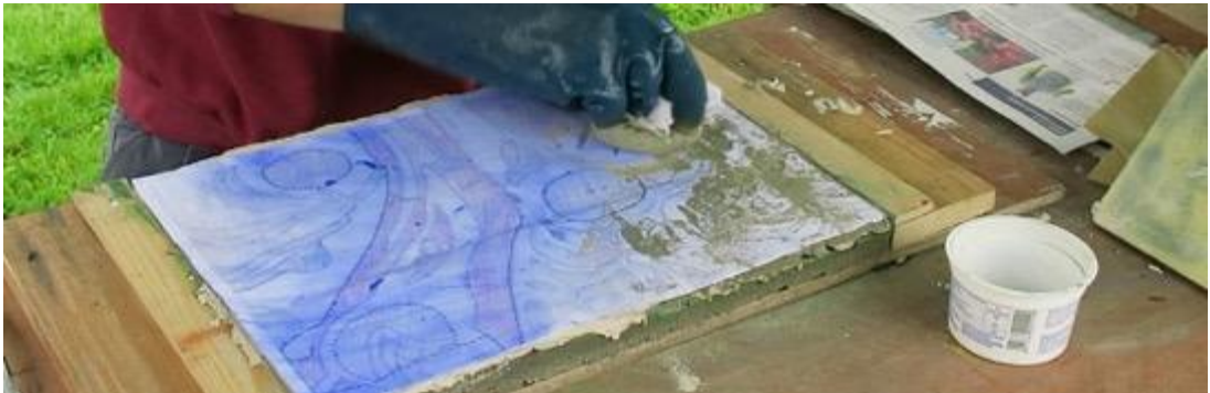
Fig. 24: Test panel 2. Pouncing through with cement in muslin bag: cement can be seen picking up moisture from the plaster below.
