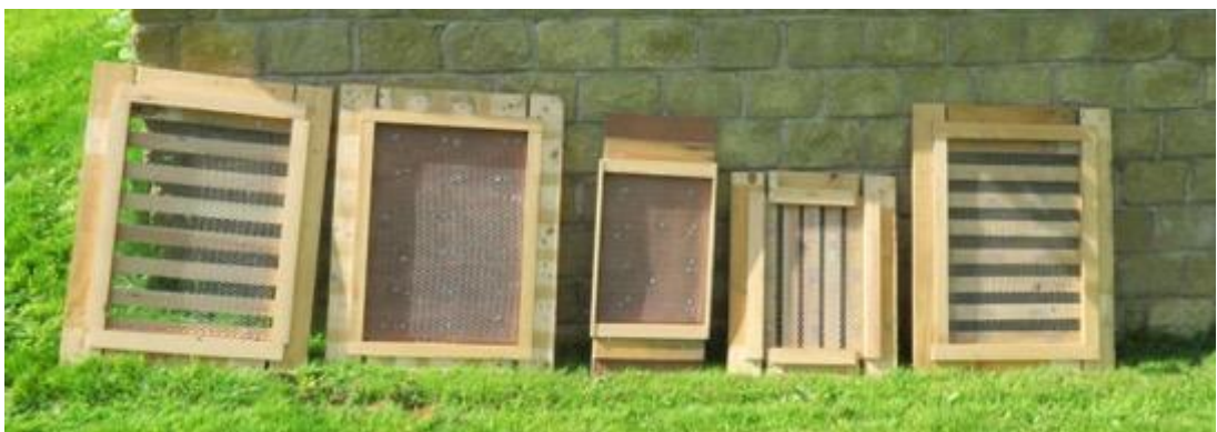
Fig. 3: Two A3 and three A2 frames made up for sgraffito tests. The difference in backing was to see if there was any impact on drying of the base coat but none was observed.
