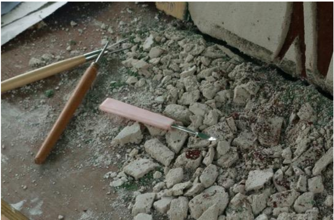
Fig. 31: The three main tools used in cleaning off remaining plaster from colour areas. From left: pottery wire loop, blunt ended bradawl and dished pewter working tool.
