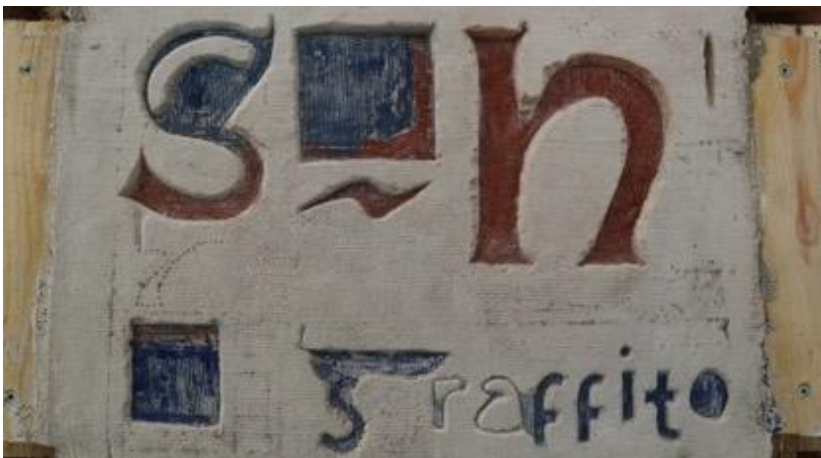
Fig. 17: Test panel 1. Extent of cutting after 2 ½ hours through crumbly stage with colours cleaned up. Note the loss of plaster above the small 's', and the rough edges, especially where the curve of the 'H' meets the upright. The large 'S' was cut as a freehand experiment without a pounced line to follow.
