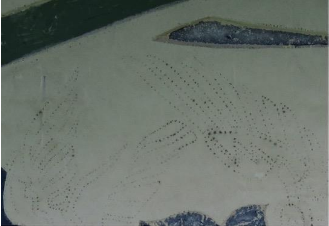
Fig. 40: Test panel 3. Completed pouncing through. The image conveys the variation in transfer of the design to the plaster but there was enough registered to make working the design accurately possible. An experiment is needed doing this with the panel vertically as Sumner would done onto church walls.
