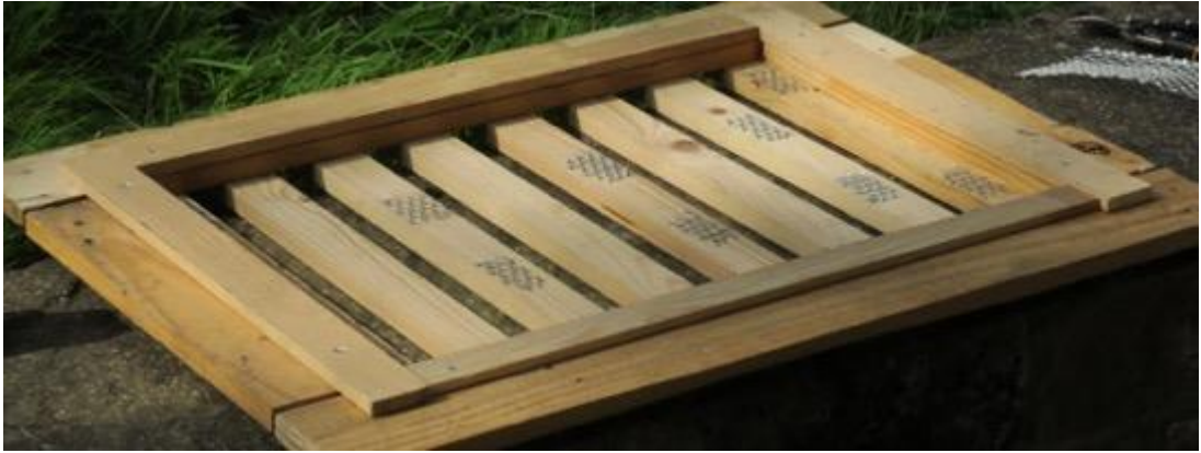
Fig. 4: A2 frame under construction showing spacers to receive mesh sheet and battens on top of the frame to define backing and topcoat thicknesses as suggested by William Millar.
