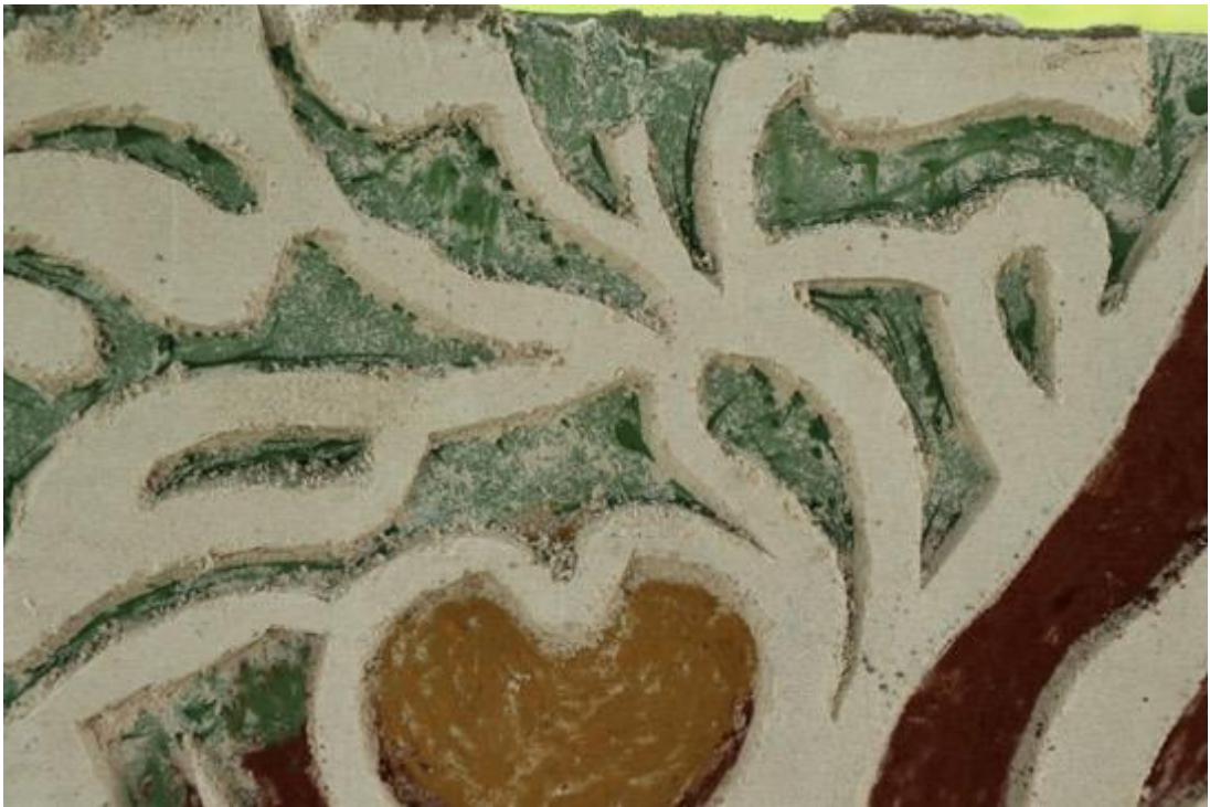
Fig. 29: Test panel 2. Initial cutting out of leaves and fruit on test panel 2 before cleaning off the coloured surfaces.
