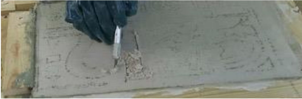
Fig. 15: Test panel 1. Starting to cut the large letter 'H' with a scalpel blade in a proprietary handle.
