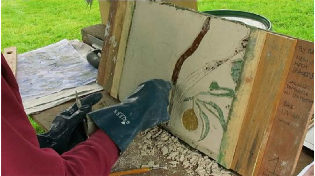
Fig. 26: Test panel 2. Cleaning off plaster residue with a wire potter's tool.
