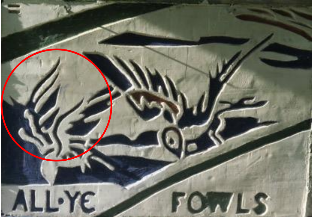
Fig. 42: Test panel 3. Finished panel with damage. This is very noticeable in the letters but also in sections ringed on the left-hand bird where creative liberties had to be taken to rescue the design, merging two feathers into one. The same problem is evident on the right-hand bird. The letters were cut at roughly hourly intervals and all except the 'Y' and 'L' presented difficulties; they should probably all have been cut in the late 'tough' stage.
