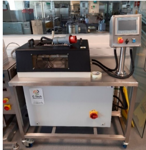
Figure 15. Image of the C-Tech Innovation batch Ohmic heater used in model validation.
