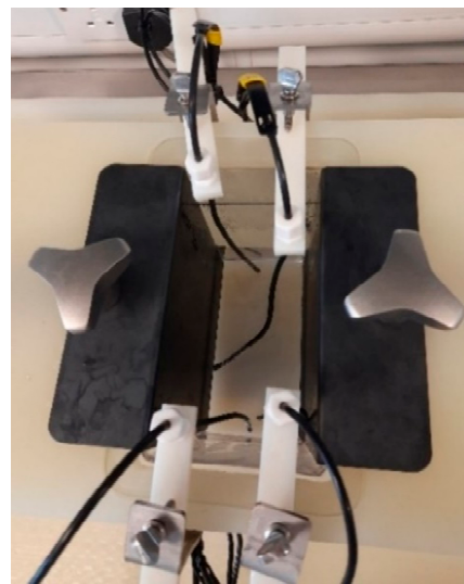
Figure 16. Heating chamber consisting of the heating cell, Ti electrodes, and 4 mounted thermocouples.
