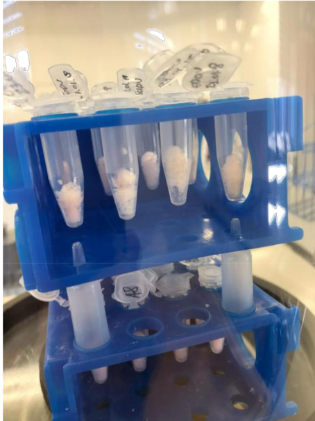
Figure 7. Lyophilised SARS-CoV-2 PV pellets within the sample drying chamber
