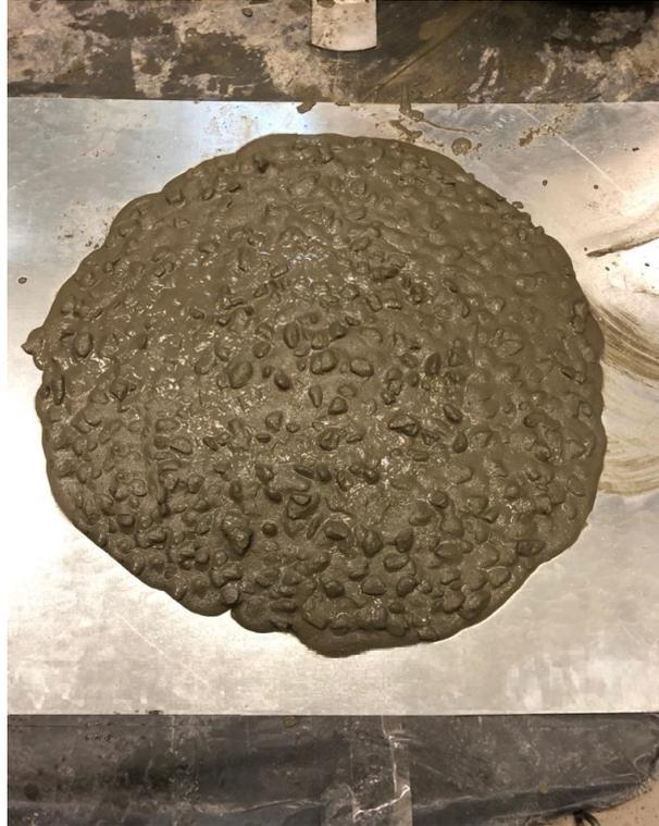
**Figura 13 – Ensaio de Slump Flow Test.**
