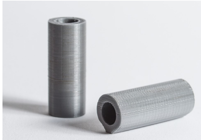
Figure 4.3: Two identical cylinders printed at the same layer height in different orientations (left: vertically, right: horizontally) 3dhubs.com/knowledge-base/how-does-part-orientation-affect-3d-print/
