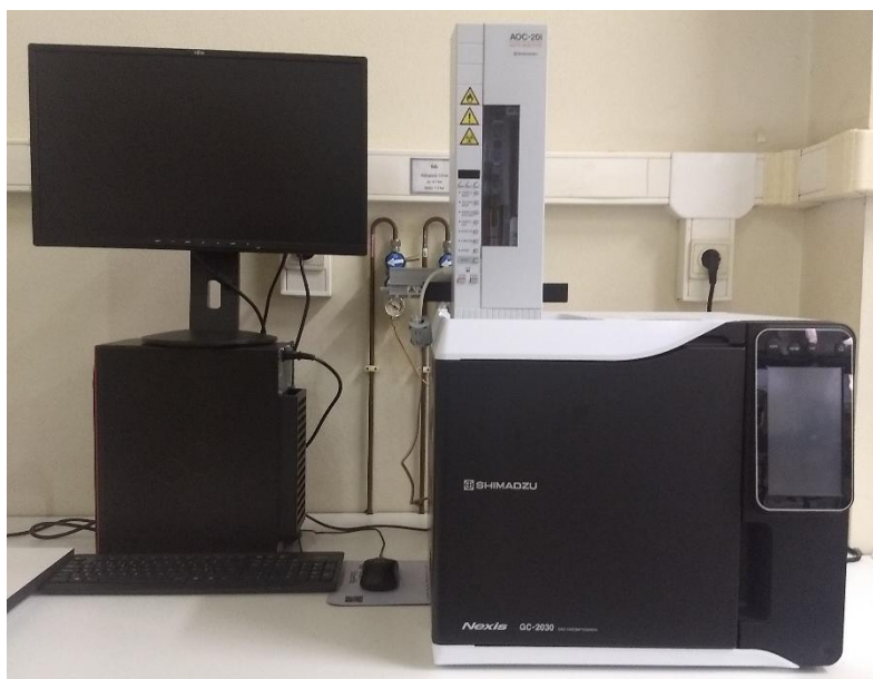
Figure 9. GC-FID equipment used for FAME analysis in biodiesel samples.
