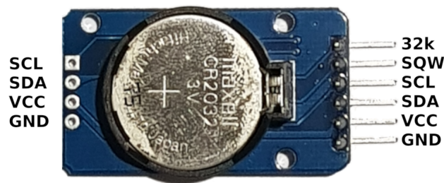
Figure 2.6: Pinout and appearance of the RTC module - DS3231
