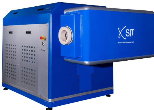
FIG. 17. Photograph of the ElectronFlash robotized system. The FLASH linac is located inside the movable irradiation head.
