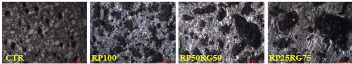
Figure 5. 16x magnification optical micrographs of printed samples
