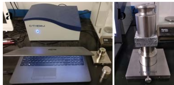
Figure 2. Thermal characterization of rubber-cement samples: C-Therm TCi analyzer (a), and test configuration (b).
