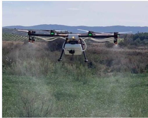
Figure 1.5. Drones used as a tool for the spread of residual-acting insecticides in the fight against mosquito.
