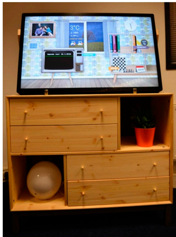
Figure 1. The eWALL home device, with a 40'' touch screen presenting the user interface, mounted on a cabinet that hides essential hardware.
