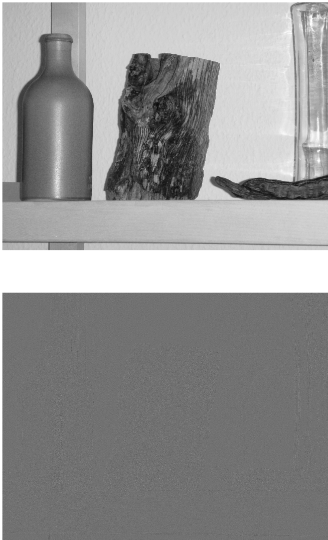
Fig. 2 Example of denoising artifacts in the residual image: top ) candidate image; bottom ) residual image computed as in eq. (2).
