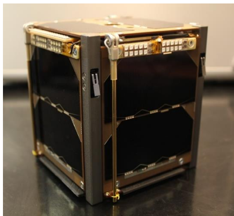
Figure 2: the LEDSAT 1U CubeSat. The LED boards on the solar panels are visible in the picture.
