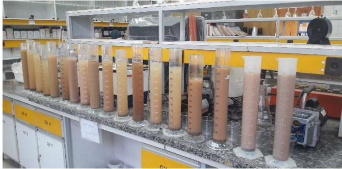
FIGURE 118 Hydrometer method to determine Soil Texture (June 2018-analyze and photo by Mahnaz Sarlak)
