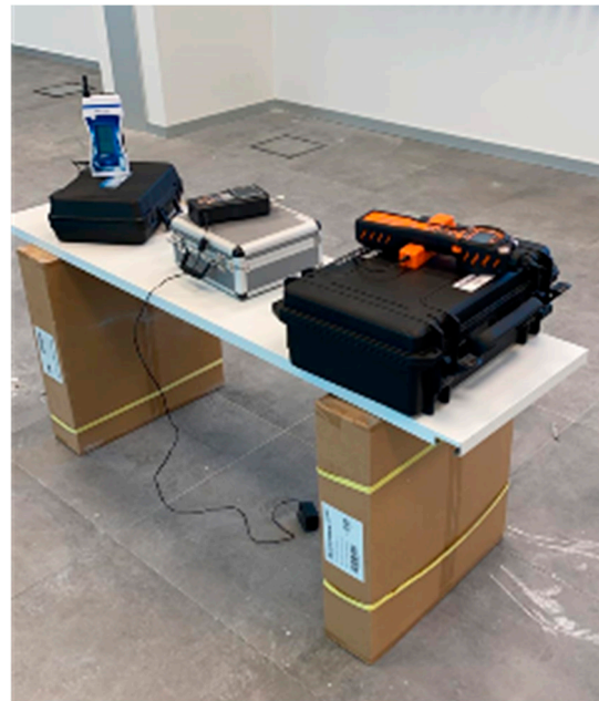
Figure 2. Sampling instruments: Multisensor 8-Channel Indoor Air Quality (IAQ) Monitor, Laser Particle Counter, Multisensor 8-Channel IAQ Monitor.
