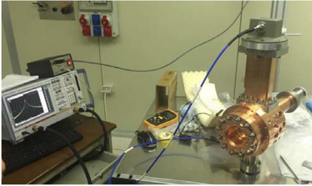
FIG. 16. Picture of the gun during low power rf tests at LNF-INFN.
