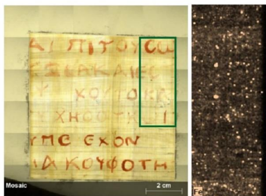
Figure 4 XRF map for iron collected using Tornado M4 spectrometer. Beam size: 50 \mu\text{m} , voltage: 50 kV, current: 600 \mu\text{A} 160 .
