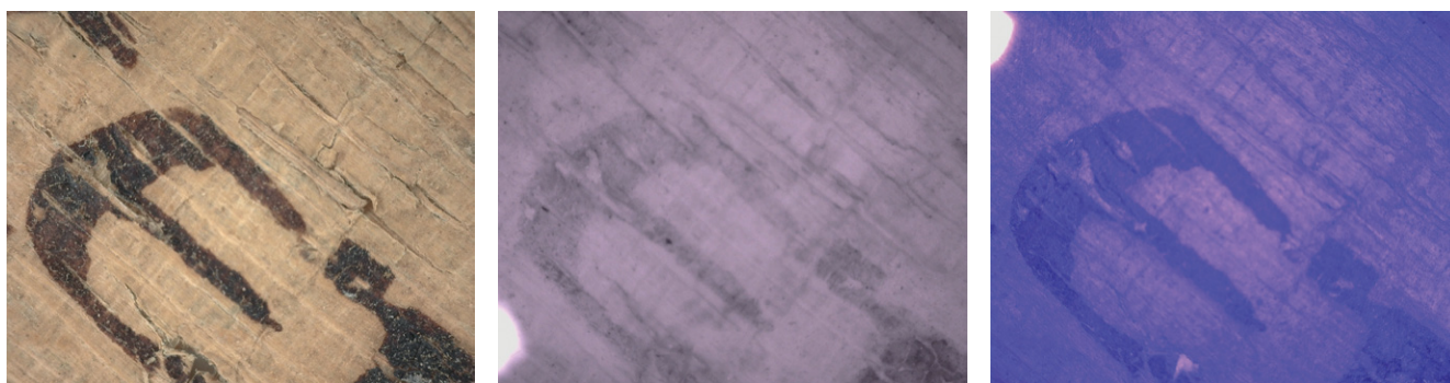
Fig. 2: Sahidic papyrus fragment Ms. Thompson HT 110.1. Fig. 2a (top): Intensities of the ink components extracted from an XRF line scan across the letter shown in the bottom images. Figs 2b, 2c and 2d (bottom): micrographs under white (left), near-infrared light (middle), and ultraviolet light (right).
