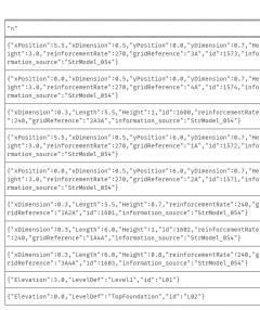
neo4;\$ MATCH (x:StructuralBeam), (y:StructuralColumn) where (x.gridReference contains y.gridReference) and (x.information\_source = y.information\_source) CREATE (x)-[r:IS CONNECTED[connectionType:'continuity'}]-(y) RETURN x, y, r
