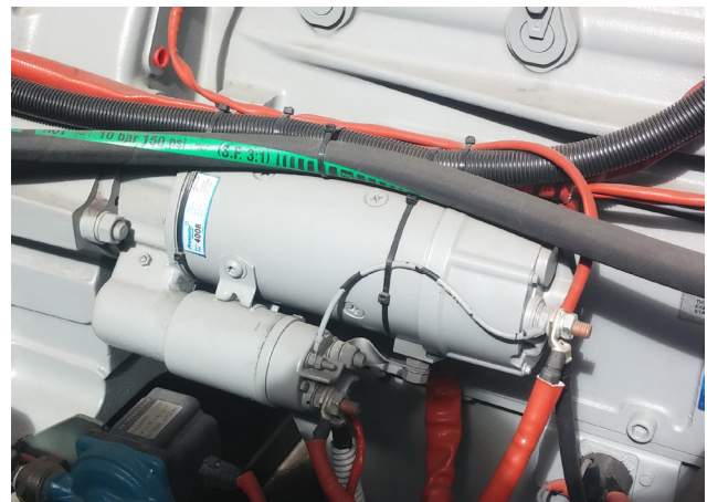
Fig. 2 Prestolite MS7-303P starter motor
