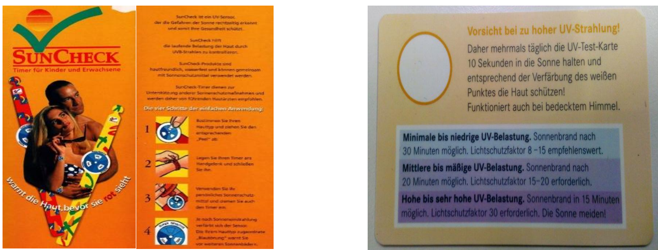
Figure 6. Examples of indicator cards (photochromic) from the 1980s and 1990s worn like a wristwatch (left) or designed like a credit card.
