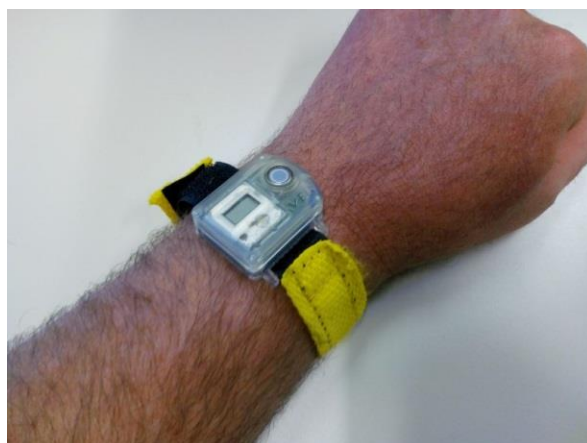
Figure 5. Miniature electronic personal irradiance meter of type SunSaver.
