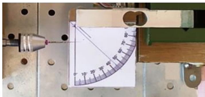
Figure 2. Mobile device with protractor for calculation of the bending angle.
