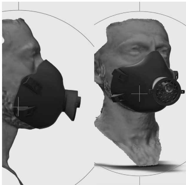
FIGURE 2. Starting from the facial scan stereo lithography interface format (STL) file an individualized facial mask is designed and melt with the STL file of the bayonet mount for the most common available filters on the market.
