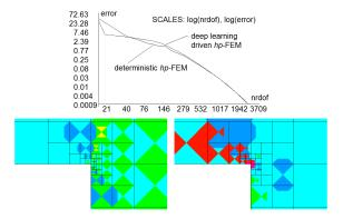
**Fig. 5.** The convergence for deterministic and DNN hp $\neg$ -FEM algorithms for the L-shape with b.c. rotated by 45 deg. The meshes of the deterministic hp-FEM algorithm and by DNN driven hp-FEM algorithm for the L-shape domain with b.c. rotated by 45 deg. Zoom  $10^5 x$  times.
